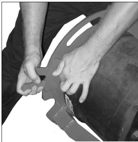
BRAKE DRUM PULLER CLOSED, LOCK BOLT AND WASHER BEING INSTALLED AND TIGHTENED
