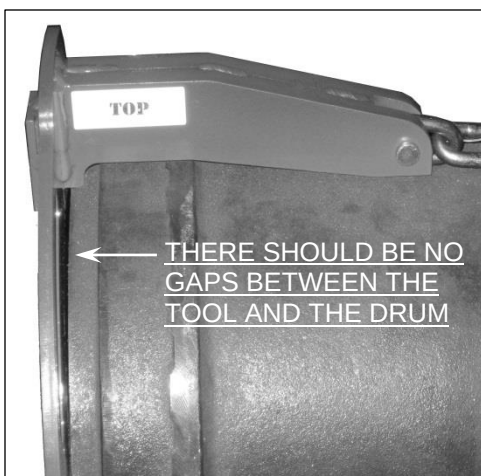
MAKE SURE THERE ARE NO GAPS BETWEEN THE BRAKE DRUM PULLER AND THE DRUM
